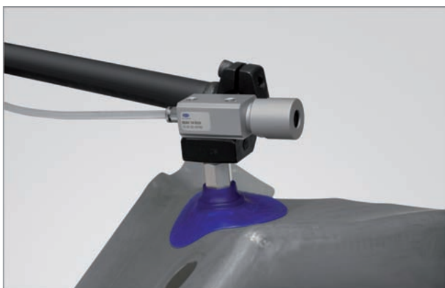
Decentral vacuum generation by ejector SEAC ECO directly at the suction pad
