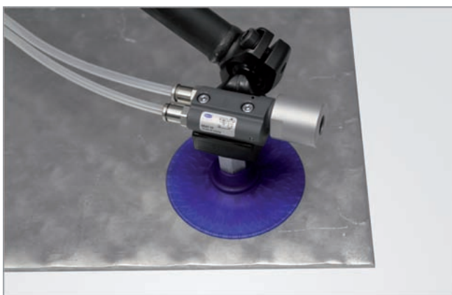
Decentral vacuum generation by ejector SEAC directly at the suction pad
